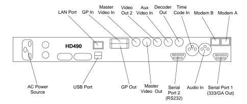
**Primary AC Power** AC power input, 120 – 240 V, 50-60 Hz tolerant. Connect to the unit's
